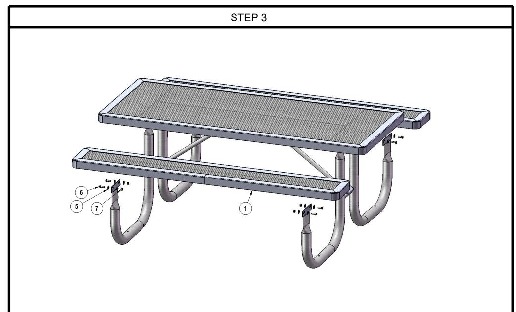
Attach the seats to the frame as shown using specified hardware.
