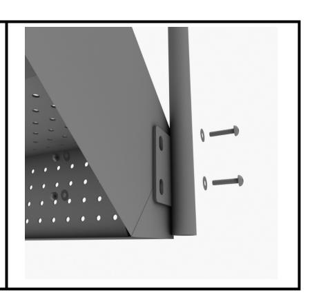
Using two (2) M10\*25 bolts, four (4) M10 washers, two (2) lock nuts, attach the handrail to the square deck.
