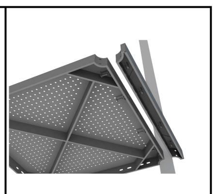
Then, See general installation guide regarding footing information for the double slide end mounts. Using two (2) M8\*20 bolts, two (2) M8 spring gaskets, and two (2) M8 washers, attach the slide end mounts to the double slide.
