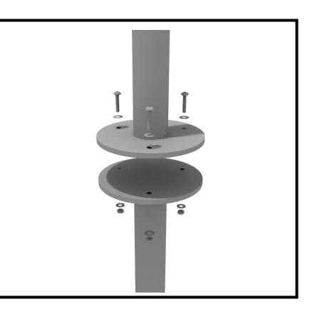
Using three (3) M10\*25 bolts, six (6) M10 washers, and three (3) M10 lock nuts, attach the pod climber to the deck.
