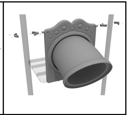
See general installation guide regarding footing information for the tube slide mount. Attach the slide end mount to the bottom of the slide using four (4) M10\*20 bolts, four (4) M10 spring washers, and four (4) M10 washers.
