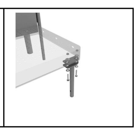
See general installation guide regarding footing information for the ADA transfer step mount. Using two (2) M10 bolts, four (4) M10 washers, and two (2) M10 lock nuts, attach the transfer step to each ADA transfer step mount.
