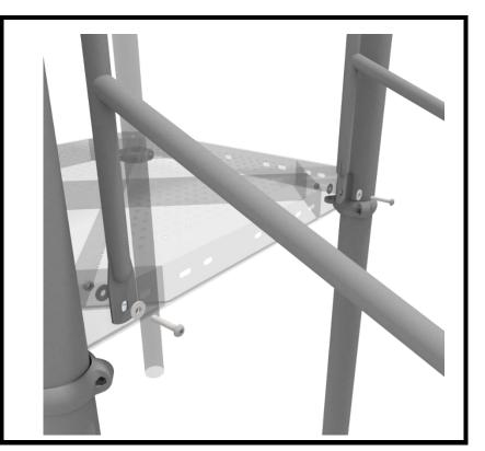
Using three (3) M10\*25 bolts, six (6) M10 washers, and three (3) M10 lock nuts, attach the ADA transfer deck to the base of the 3-foot ADA transfer stair.
