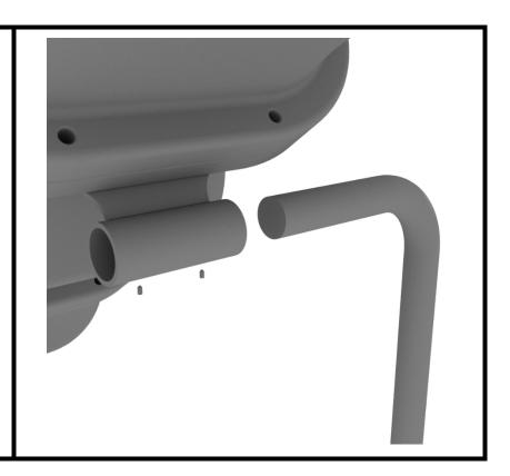
Finally, connect the tube slide together using ten (10) M8\*30 bolts, ten (10) M8 washers, and ten (10) M8 lock nuts.
