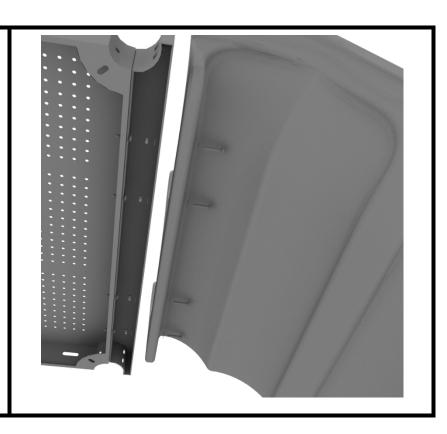
Once the slide is attached, take the double slide hood and insert hood into the top of the slide, and then attach the top using two (2) double slide clamps, and two (2) M8\*30 bolts.
