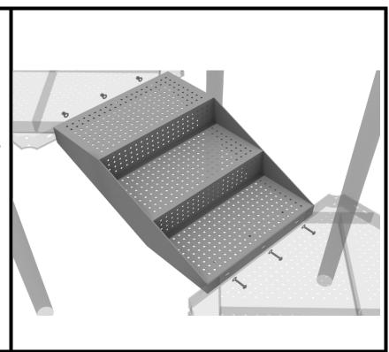
Then, once the stair is in place, attach the 12-inch connection handrail to the posts using four (4) 3.5-inch tube clamps, and four (4) M8\*30 bolts. Then, attach the bottom of the handrails to the decks using one (1) M10\*25 bolt, two (2) M10 washers, and one (1) M10 lock nut for each attachment point.
