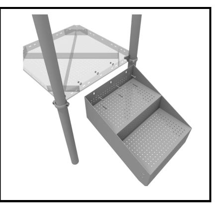
Using four (4) M10\*25 bolts, eight (8) M10 washers, and four (4) M10 lock nuts, connect the bottom of the handrails to the bottom of the 3-foot transfer stair.
