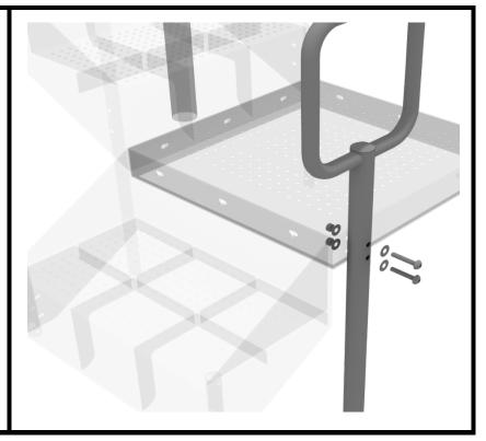
Using two (2) M10\*25 bolts, four (4) M10 washers, and two (2) lock nuts, attach the transfer deck mount to the ADA transfer deck.
