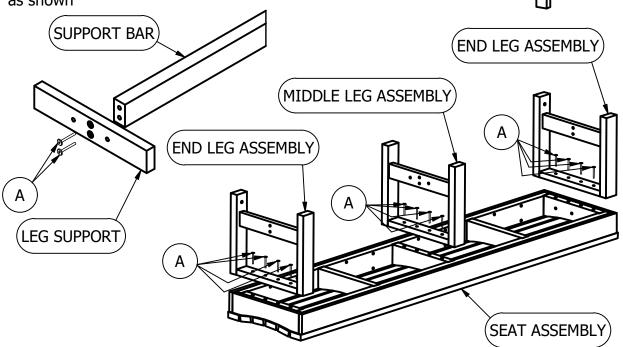
**2)** Attach Leg Assemblies to Seat Assembly using (12) "A" Bolts, Middle Leg Assembly Brace offset to left, as shown.
