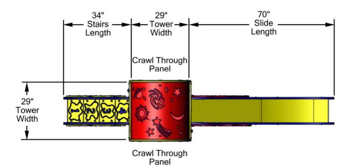
All Attachments are Modular. Attachments Can Be Placed on Any of Four Sides of Center Tower.
