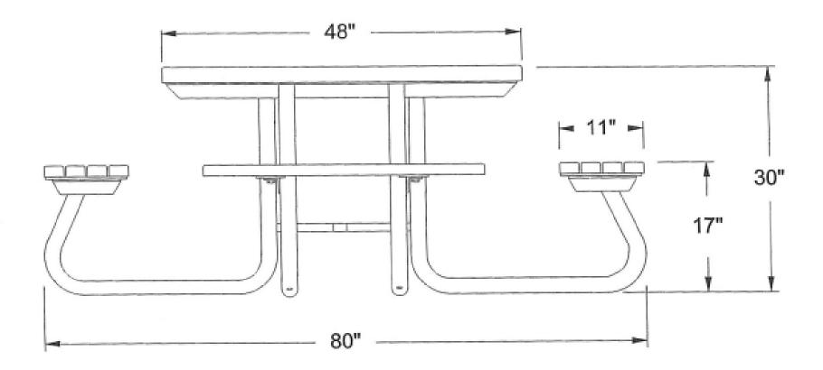
The frame is made from heavy 1 5/8" OD pipe.
